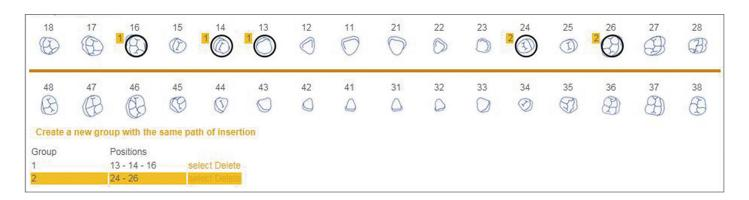
Abutments in a group with parallel alignment/same path of insertion are designated with the same number
